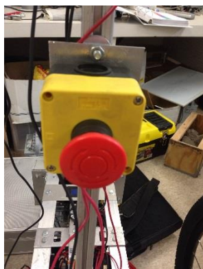
Figure 3: Physical Emergency Stop
