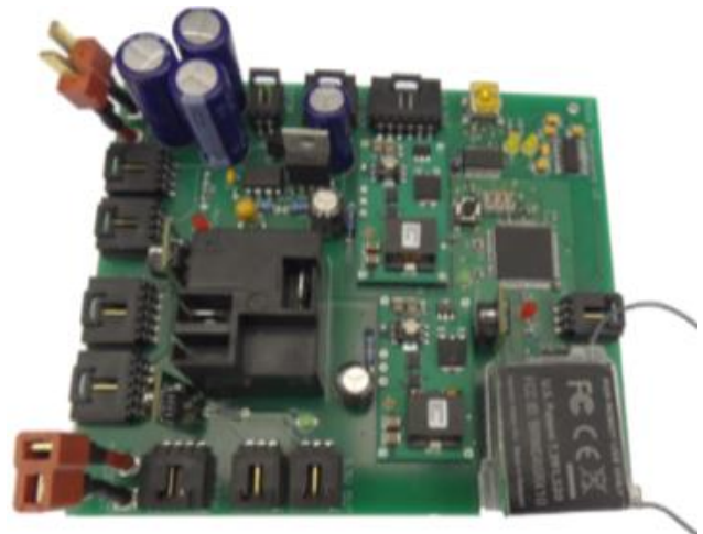
Figure 7: Zero 2 power distribution and motor control system.
