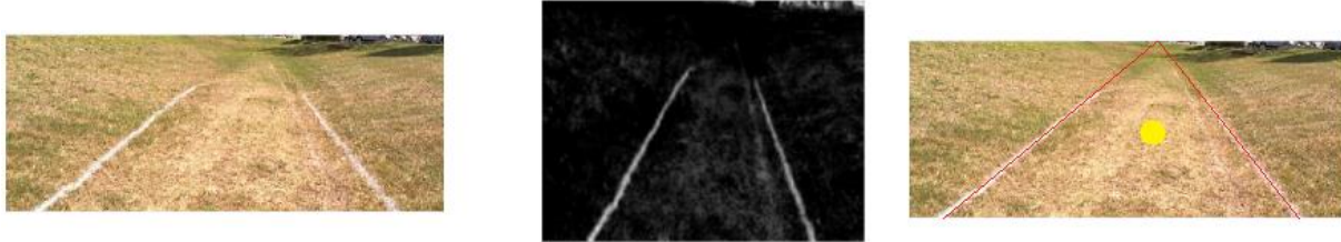
Figure 6: Image processing images where the lines are filtered out and the image is overlaid with read lines to show the actual detected lines. The yellow dot determines the heading in relation to the vehicle.
