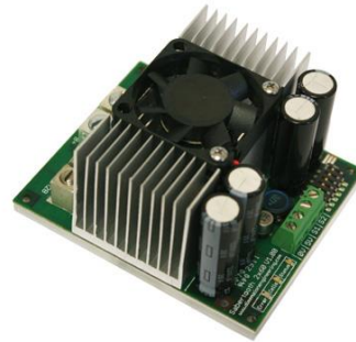
Figure 7 - Sabertooth 2x60 Dual Motor Driver
