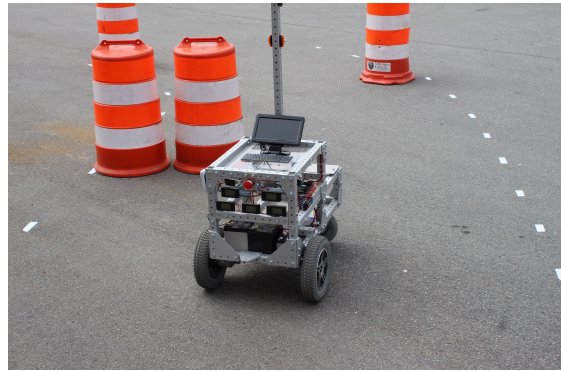
Figure 8: Picture of the platform navigating through a sample course avoiding obstacles and within the course width of 10 feet between the lines
