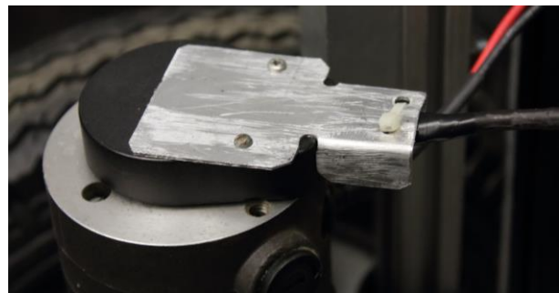
Figure 3: Motor encoder wiring protection bracket
