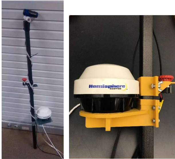
Figure 4: Sensor pole with close-up of updated 3D printed mounts
