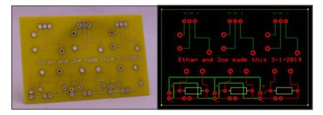
*Figure 6: Custom-designed printed circuit board + PCB routing.*
