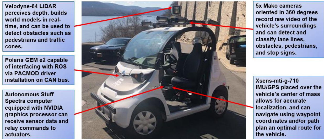
Figure 5: AVRAD's GEM e2, outfitted with the various sensors that the system utilizes to accomplish urban navigation.
