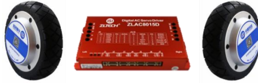
Figure 4. Adopted in-wheel motors for Orange2023.
