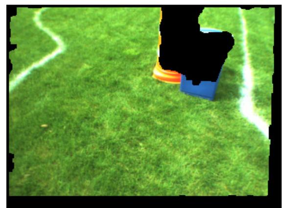
Figure 8: This figure shows the image after the obstacles have been filtered out. Note that while the filter is effective, it does miss the edges of the obstacles.
