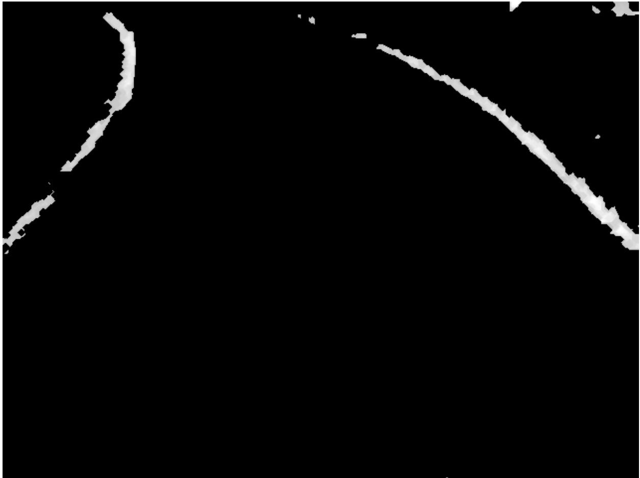
Figure 6: The results of our simple thresholding algorithm run on one of the images we took of the course last year.
