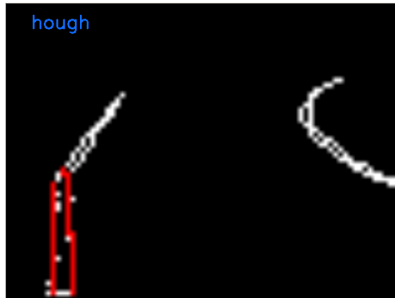
Figure 11: Applying a hough transform to detect lines.
