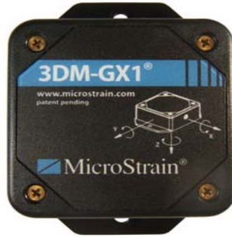
Figure 2: The 3DM-GX1 IMU. Programs are stored in non-volatile flash memory and communication with the host computer is via USB
