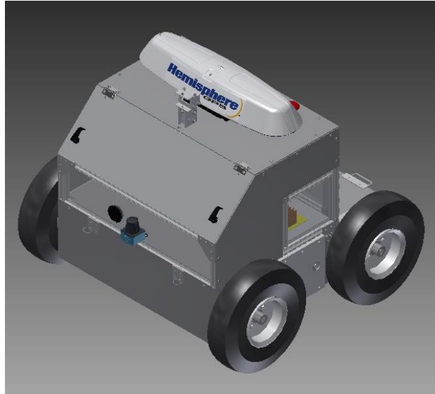
Figure 4. Top Chassis Mated to Bottom Chassis
