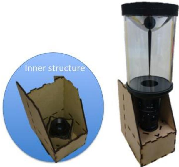
Figure 8. The New omnidirectional camera
