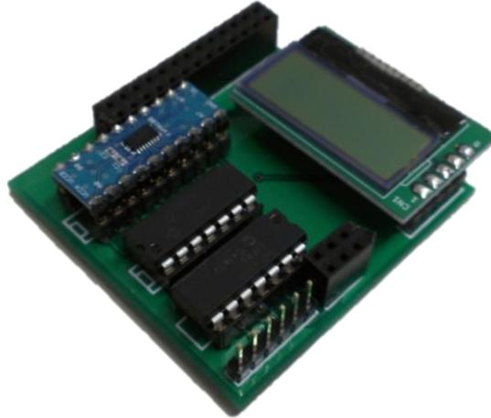
**Figure 10. AD/DA circuit used PCB**
