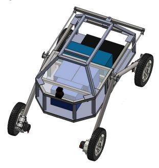
The control arm sections located on either side of the chassis are attached to the chassis with a custom made aluminum shoulder bolt. Each arm is made out of 1.5 inch steel tubing, which attaches to the wheelchair hub motors. Because of the large linear forces and torques applied to this section of the robot, this is where we most likely will have failures in our system.
