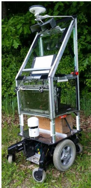
**Figure 1 - The Robotic Platform Mantis 2.0**
