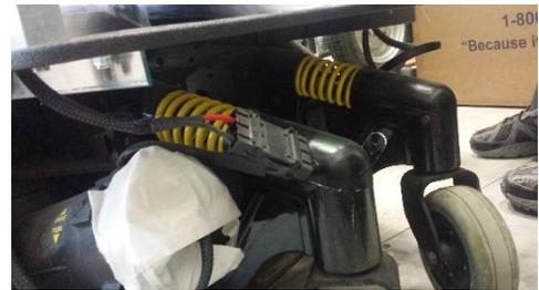
**Figure 6 - Mechanical Suspension**
