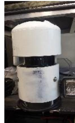
**Fig 5. Enclosed LIDAR**
