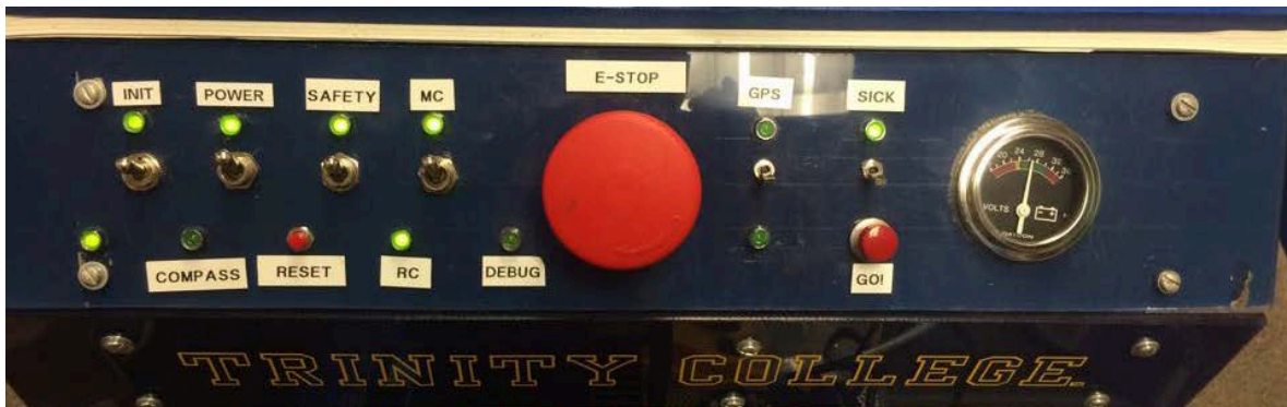
Figure 4: Q's Control Panel, located in rear of robot
