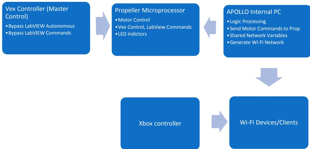
Figure 3.1 APOLLO Communication System and GUI
