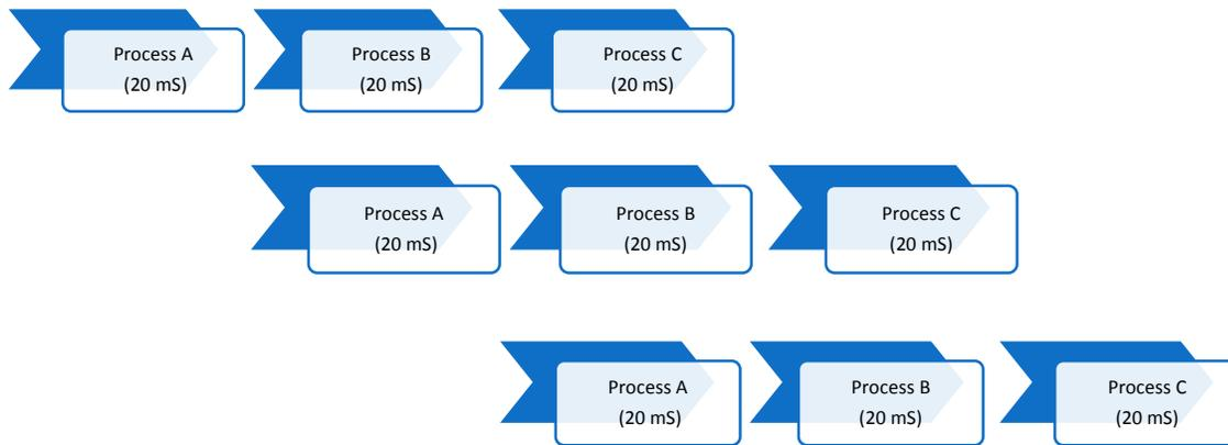
Figure 3.2 Pipelined Vision process
