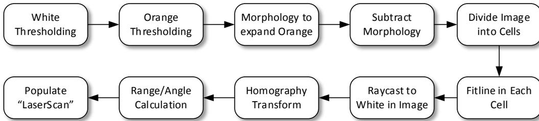
Figure 7. Image Processing Pipeline
