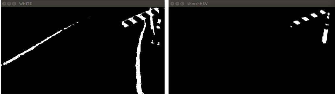
Figure 9. White Threshold (left) and Orange Threshold (right)
