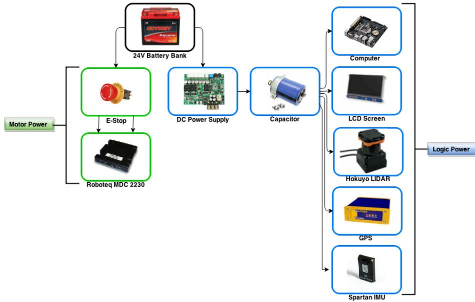
**Figure 3. Power System Distribution Block Diagram**
