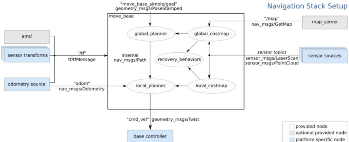
**Figure 10. ROS Navigation Stack Structure\***
