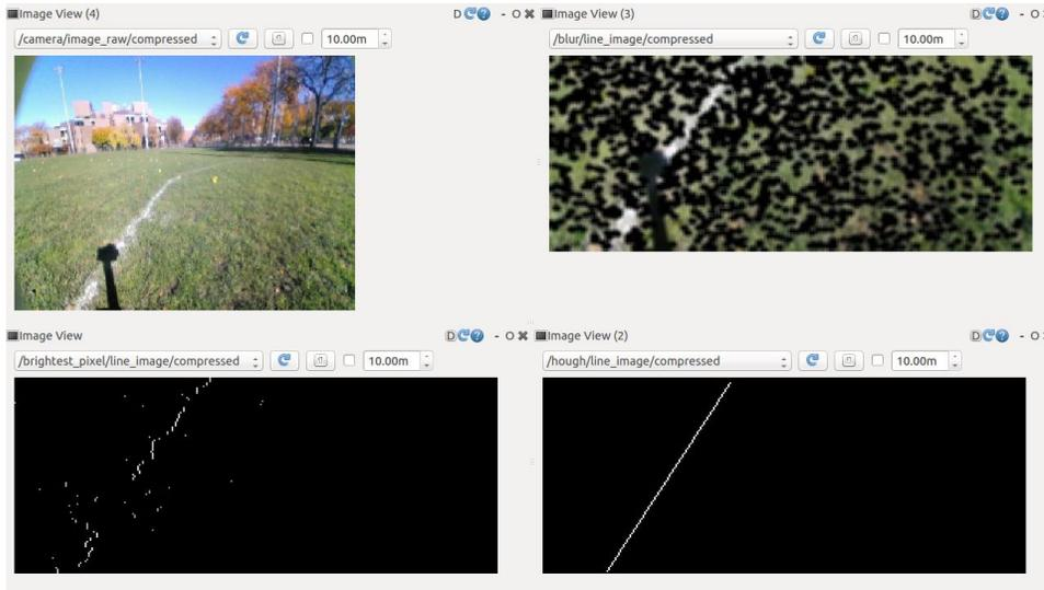
Figure 9. Debug image output of different stages of line detection algorithm. Raw camera data (top left) is backprojected then blurred (top right). Then ran through a brightest pixel filter (bottom left) and finally a Hough transform to extract the lines (bottom right).
