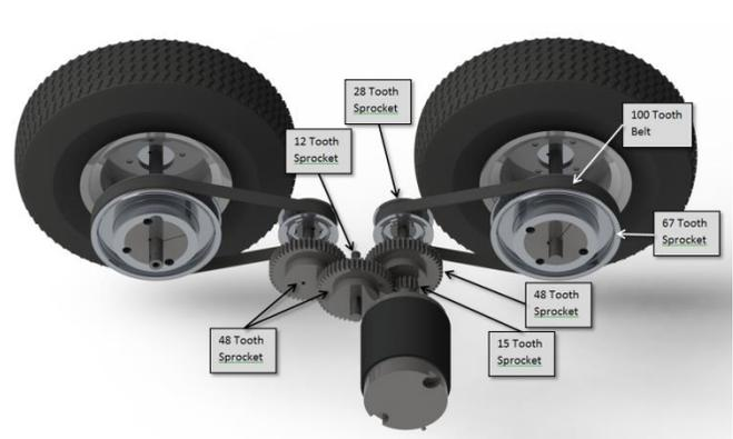
Figure 3. Gearbox Skeleton View
