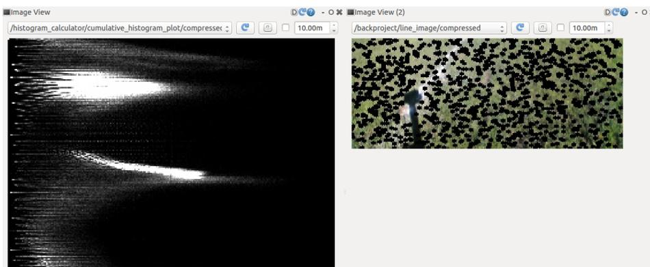
Figure 8. Heatmap of constructed histogram from training image (left), where the x axis corresponds to saturation values, the y axis corresponds to hue values, and the intensity corresponds to the relative count of those pixels. The resulting backprojected pixels are subtracted from the camera input during a run, removing a lot of noisy grass areas (right).
