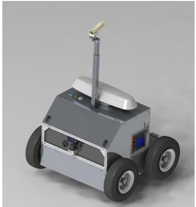
Figure 4. Top Chassis Mated to Bottom Chassis
