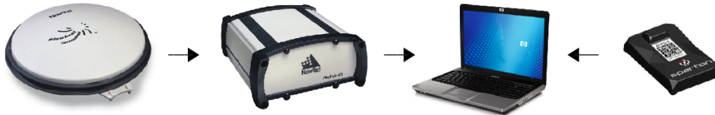
Figure 16: Navigation flowchart [from left to right: GPS antenna, GPS receiver, computer, compass]
