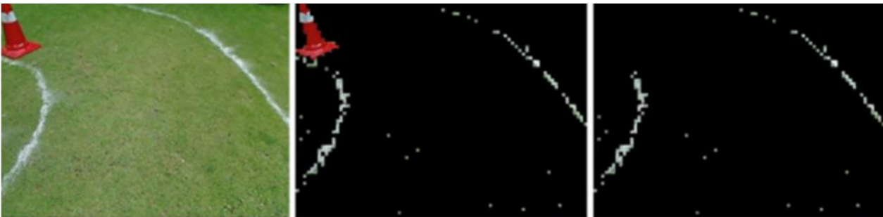
Figure 19. Output at different steps, from original image (left) to grass Removal (centre) and obstacle removal with lidar data (right)
