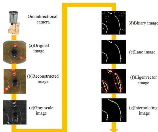
**Figure 17. Lane detection procedure**
