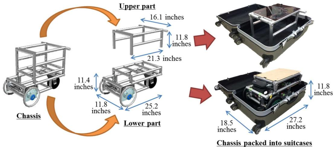
**Figure 4. Lower and upper parts of chassis packed into suitcases**
