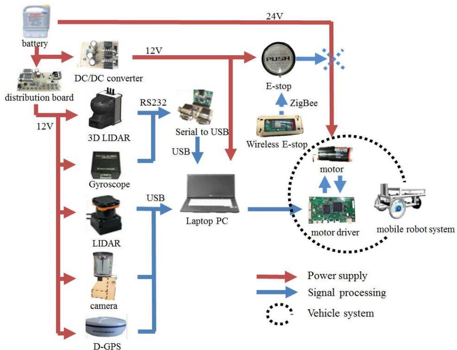
**Figure 12. Electrical power and signal configuration of Orange 2015**
