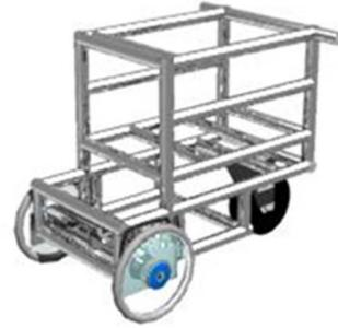
**Figure 9. CAD of Orange2015 chassis**
