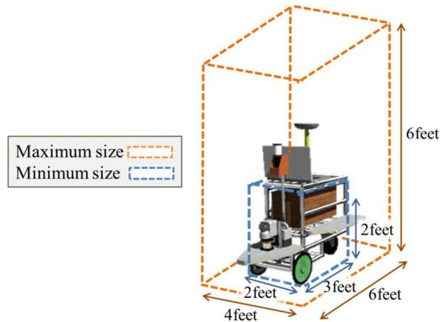
**Figure 6. Size comparison between IGVC rules and Orange2015**
