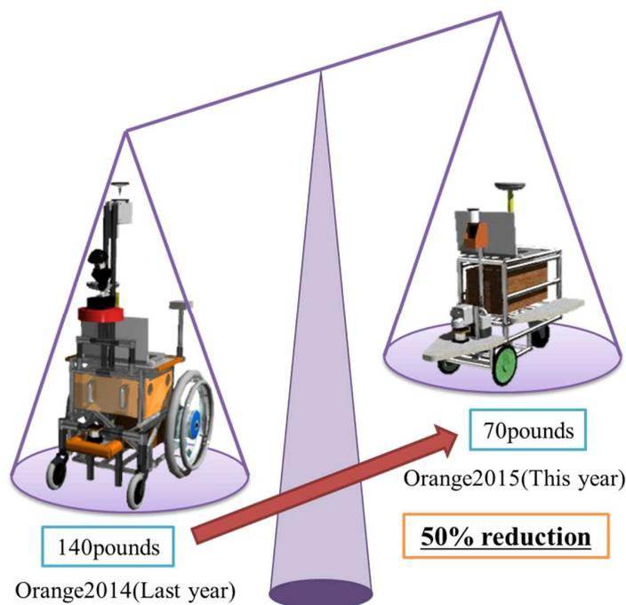
**Figure 7. Weight comparison between Orange2014 and Orange2015**
