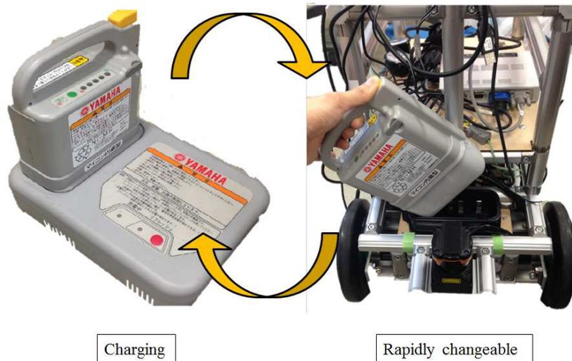
**Figure 11. Rapidly changeable batteries**
