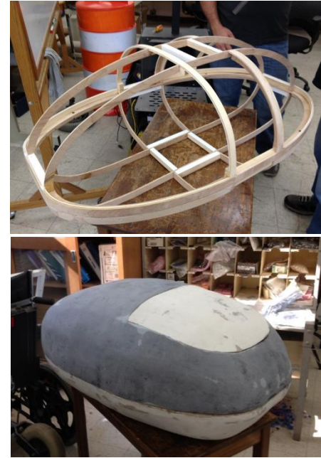
Figure 9: Top: Apollo II's Wooden Frame; Bottom: Fiberglass Exterior is Added
