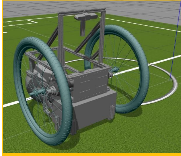
Figure 7.3: Model can be used to put accurate sensor locations on robot
