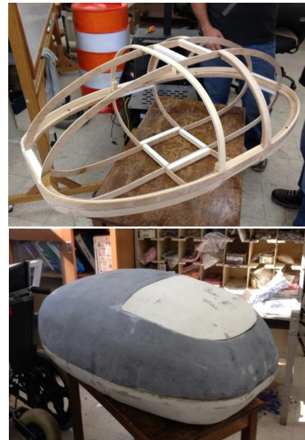
Figure 3: Top: Apollo IV's Wooden Frame; Bottom: Fiberglass Exterior is Added
