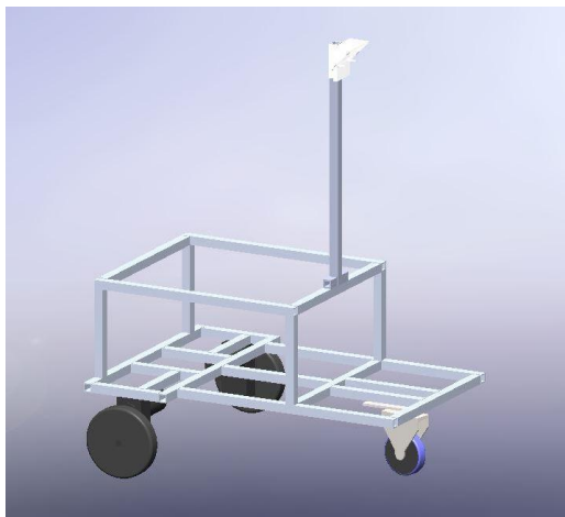
Figure 3: Space frame with wheels attached
