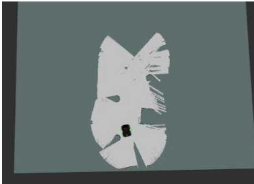
Figure 12 GMapping with LiDAR Points
