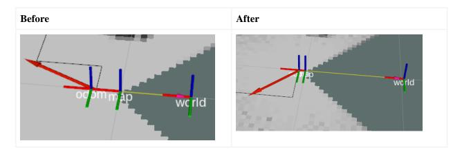
Before path planning is performed, a costmap is generated by applying OpenCV's dilation operation to the map. This ensures any valid path will have a buffer distance of about 0.5m to the nearest obstacle.
