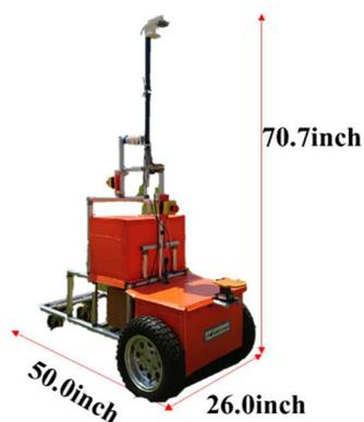
**Figure 5. The Orange 2019 vehicle body**
