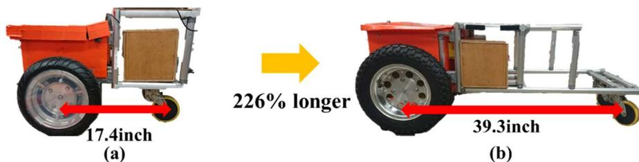
**Figure 8. Distance from front and rear axle (a)before, (b)after**
