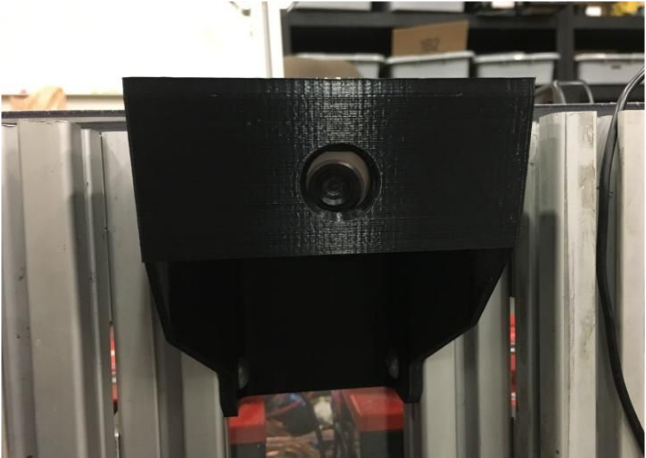
The LiDAR mount, which houses the front-facing camera.
