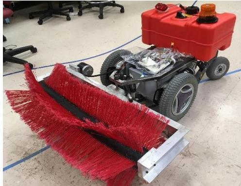
Figure 1. Autonomous snow removal robot
