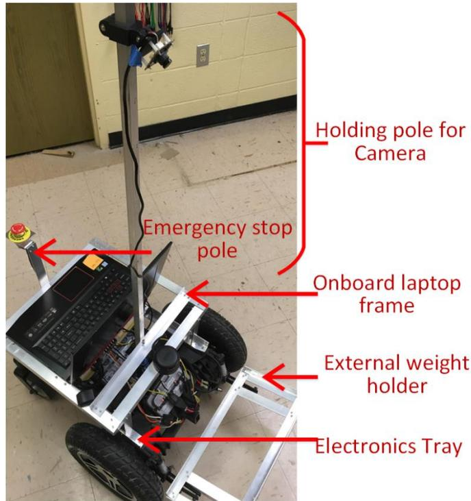
Figure 2. Overview of the mechanical structure of the macro mouse
