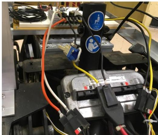
Figure 3. H-bridge to motor connections during testing
