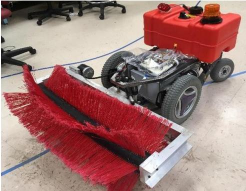
Figure 1. Autonomous snow removal robot
