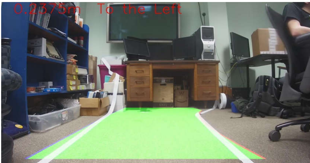
Figure 5 – Lane Detection with Adequate Curve Fitting for Solid Lines
