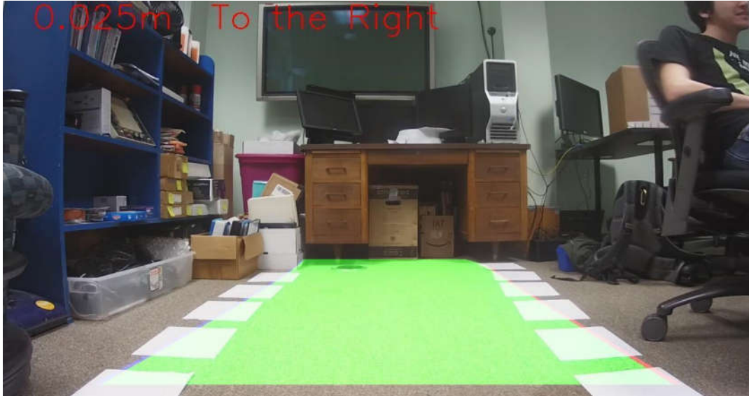
Figure 6 – Lane Detection with Broken Lines
