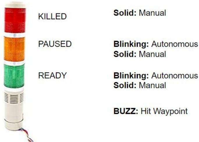
**Figure 6: Tower light operation**
