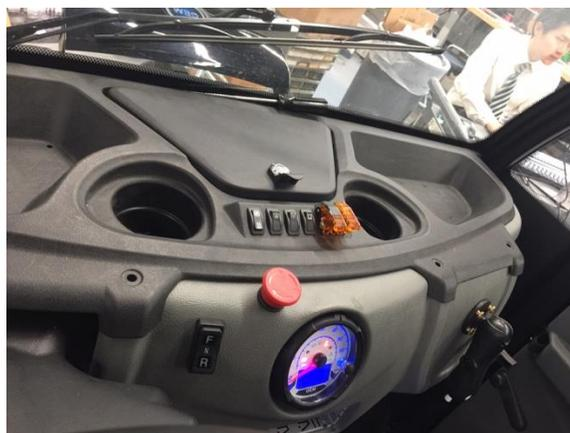
Figure 27: Dash Emergency Stop and Power Switches
