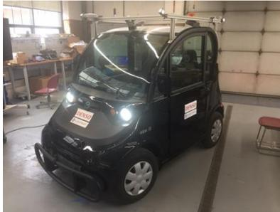
Figure 2: Polaris Gem e2 with frame and sensors
