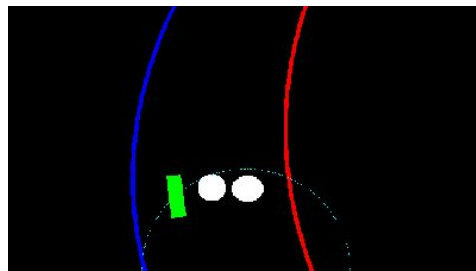
Waypoint generation [blue and red lanes, white obstacles, green robot]
