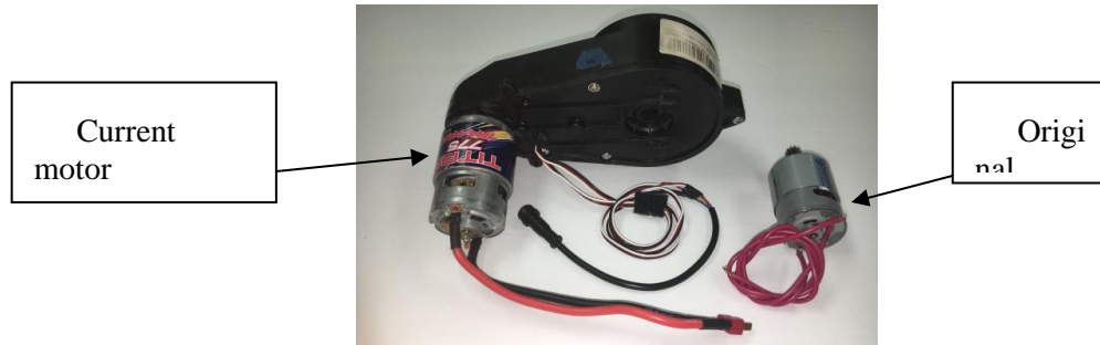
Figure 6. Drive mechanism with larger motor (gearbox + motor).
