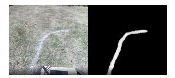
FIG. 12: Cropped example showing the output of our U-Net on an image.
