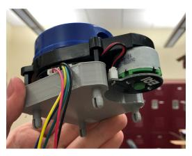
FIG. 4: 3D printed LiDAR mount easily attaches to the polyboard shelf.
