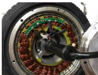
Figure 3: Image of Brushless hub motors used in the drivetrain
