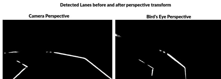
Figure 12: Detected Lanes before and after perspective transform
