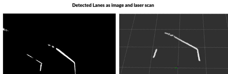
Figure 13: Detected Lanes as Image and Laser Scan
