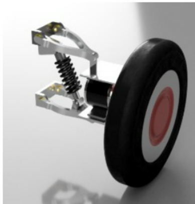
Figure 4b: Drive wheel suspension
