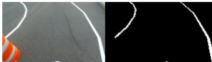
(left) Original image, (right) output of the thresholding method
