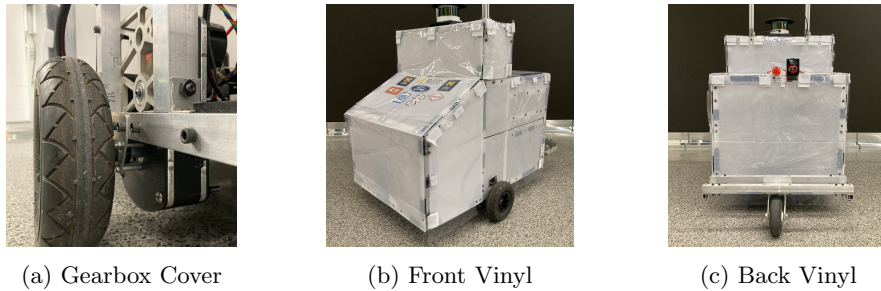
Figure 8. Dry and Wet Vehicle Weatherproofing Measures
