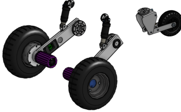
Figure 5: Isolated view of front and rear suspension systems
