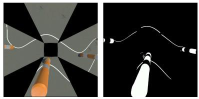
*Twistopher* uses a classical computer vision approach to transform our four video streams into an obstacle map that the vehicle can use to navigate. First, the images are passed through correction filters to correct for camera warp and to project the image onto a 2D plane. Then, the images pass through a series of filters that turn the images into obstacle maps. Finally, the four separate obstacle maps are overlaid to create a
