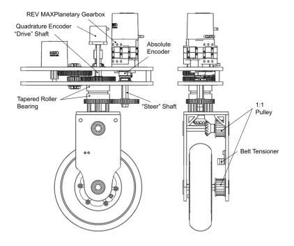
angle of the module between power cycles. Each swerve module features an 8-inch pneumatic wheel, which is ideal for all-terrain and all-weather performance. The modules are designed such that the gearbox is attached to the frame of the robot, so that the modules can be easily removed and installed independently of the gearboxes. This allows for easier assembly and transport, and we can have a spare module fully assembled on standby in case any need to be quickly replaced.
