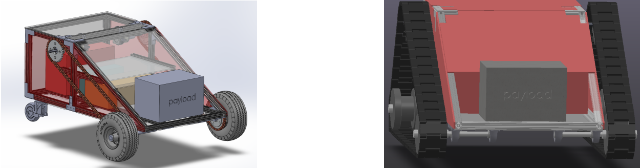
Figure 1: Left: Scarlet Rover configured with wheels. Right: Scarlet Rover with tracks installed.
