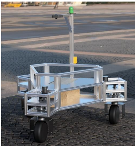
Fig 2.1 Warrior 1 three-wheel swerve-drive mechanical layout
