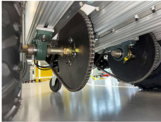
Figure 2 - ATNA drivetrain showing the independent axle section, chain drive, sprockets, pillow block bearings, and drive wheel.
