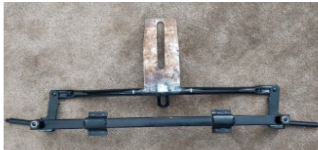
Figure 4: Steering system with extended lever arm.
