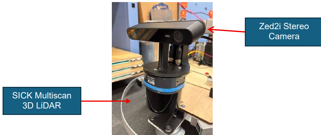
Figure 8: ZED2i Camera and SICK Multiscan 3D LiDAR
